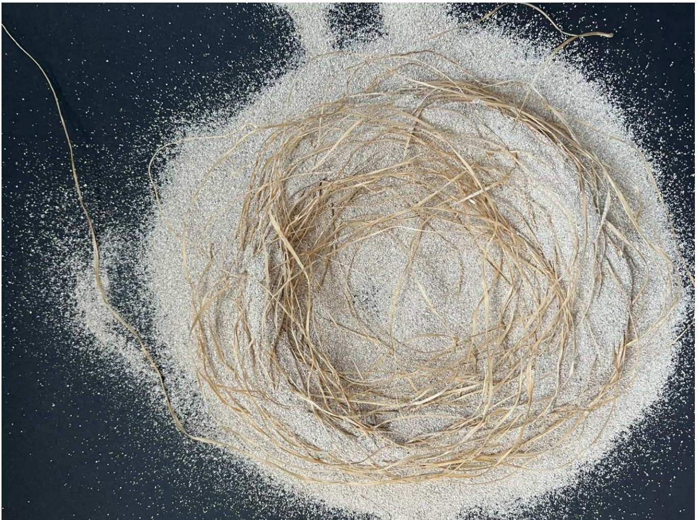
FIG 12. THE COIL IS CONTROLLED BY A SMALL LAYER OF SAND, PREVENTING THE COIL FROM TANGLING DURING TWISTING. PHOTO BY MARIE WALLENBERG.
