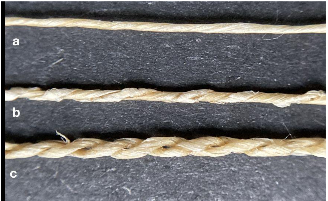
FIG 15. COMBINATIONS OF SPLICING POINTS IN ONE OF THE FINISHED 2-PLY YARNS MADE DURING THE EXPERIMENTS. TOP: TWISTED YARN CONSISTING OF TWO FIBRE RIBBONS APPEARING ALMOST AS A 1-PLY THREAD (A); MIDDLE: TWISTED YARN CONSISTING OF A FIBRE RIBBON AND ONE SPLICING POINT (B); BOTTOM: TWISTED YARN CONSISTING OF TWO SPLICING POINTS BEING TWISTED TOGETHER, PRODUCING A SECTION WITH HIGH TWIST (C). PHOTO BY MARIE WALLENBERG.
