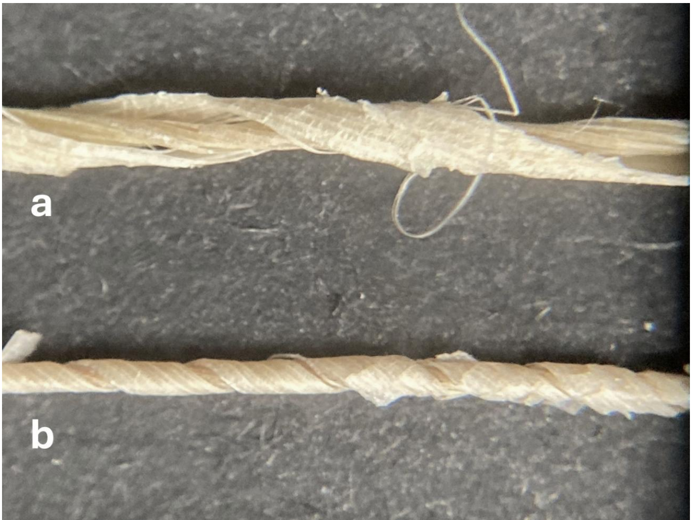
FIG 6. FLAX RIBBONS SPLICED WITH (A) NARROW ANGLE BETWEEN THE FIBRE RIBBONS AND (B) WIDE ANGLE BETWEEN THE FIBRE RIBBONS. PHOTO BY MARIE WALLENBERG.
