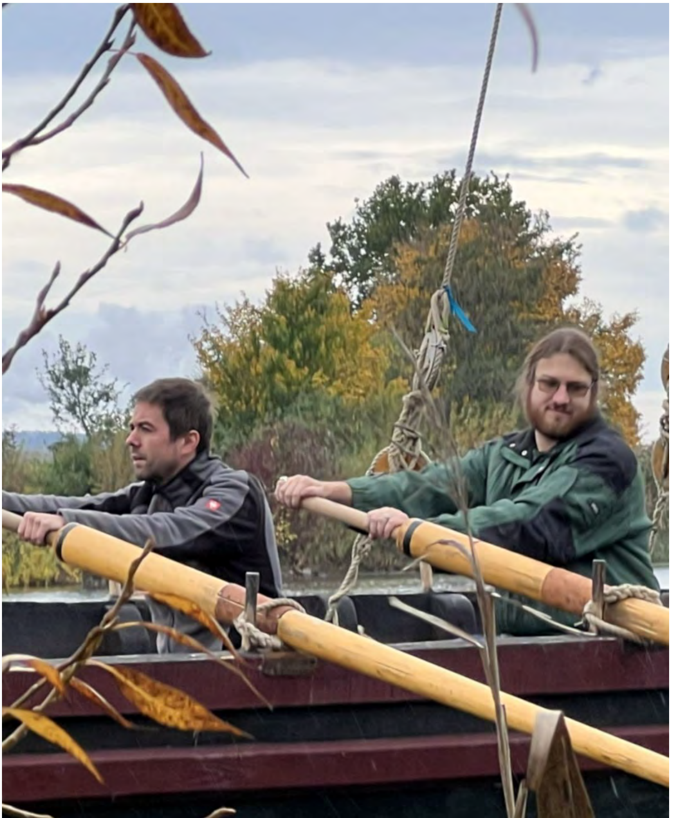
FIG 5B. THE DIFFERENT BELT SUSPENSIONS ARE SHOWN HERE, THE HISTORICAL SUSPENSION (EVIDENCED BY ABRASION AT THE THOLEPINS OF THE BOAT WRACKS) WITH A ROPE RING (STROKE). PHOTO BY B. DREYER
