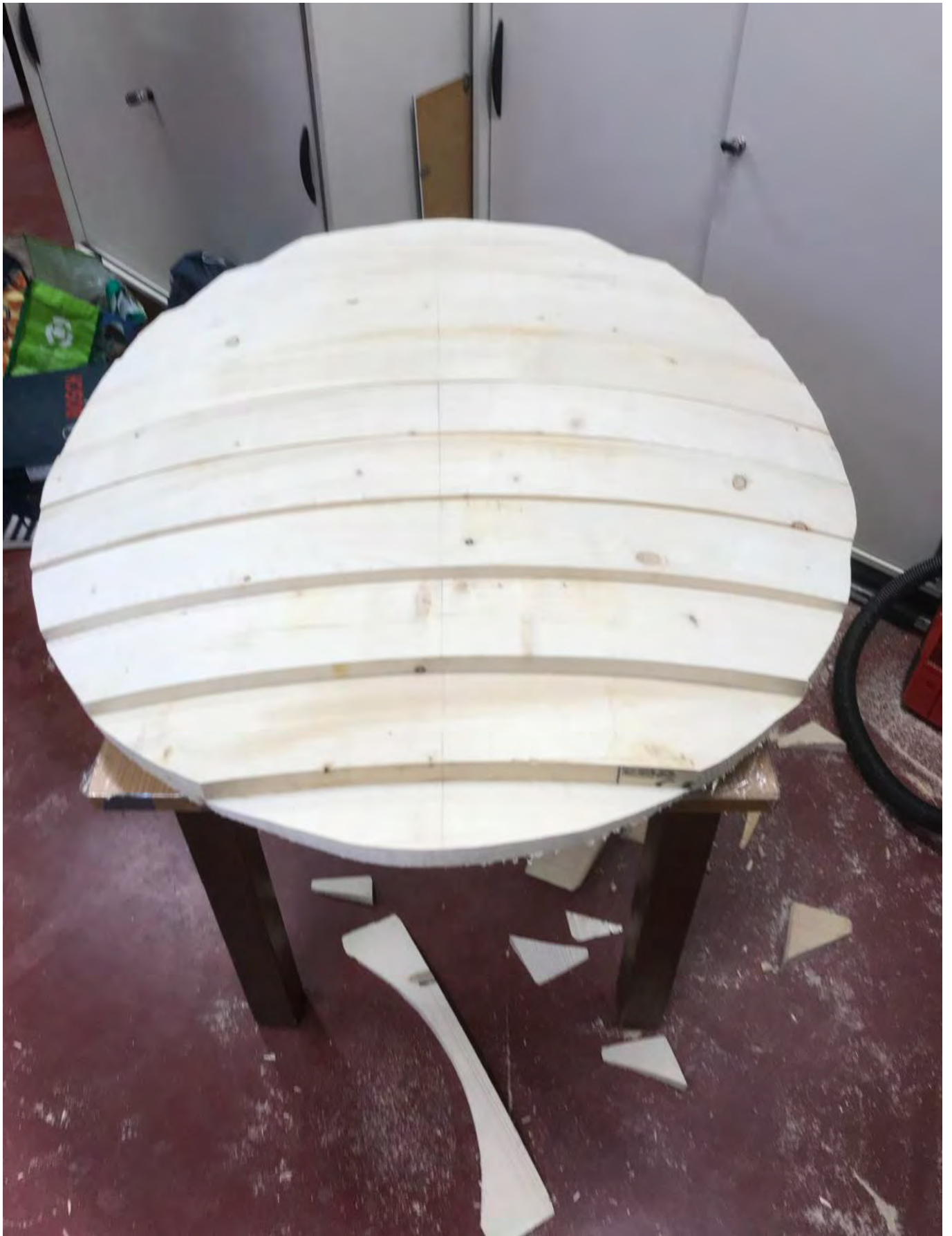
FIG 33. SHIELD TEMPLATE (MASSIVE PINE) UNDER CONSTRUCTION. PHOTO BY B. DREYER
