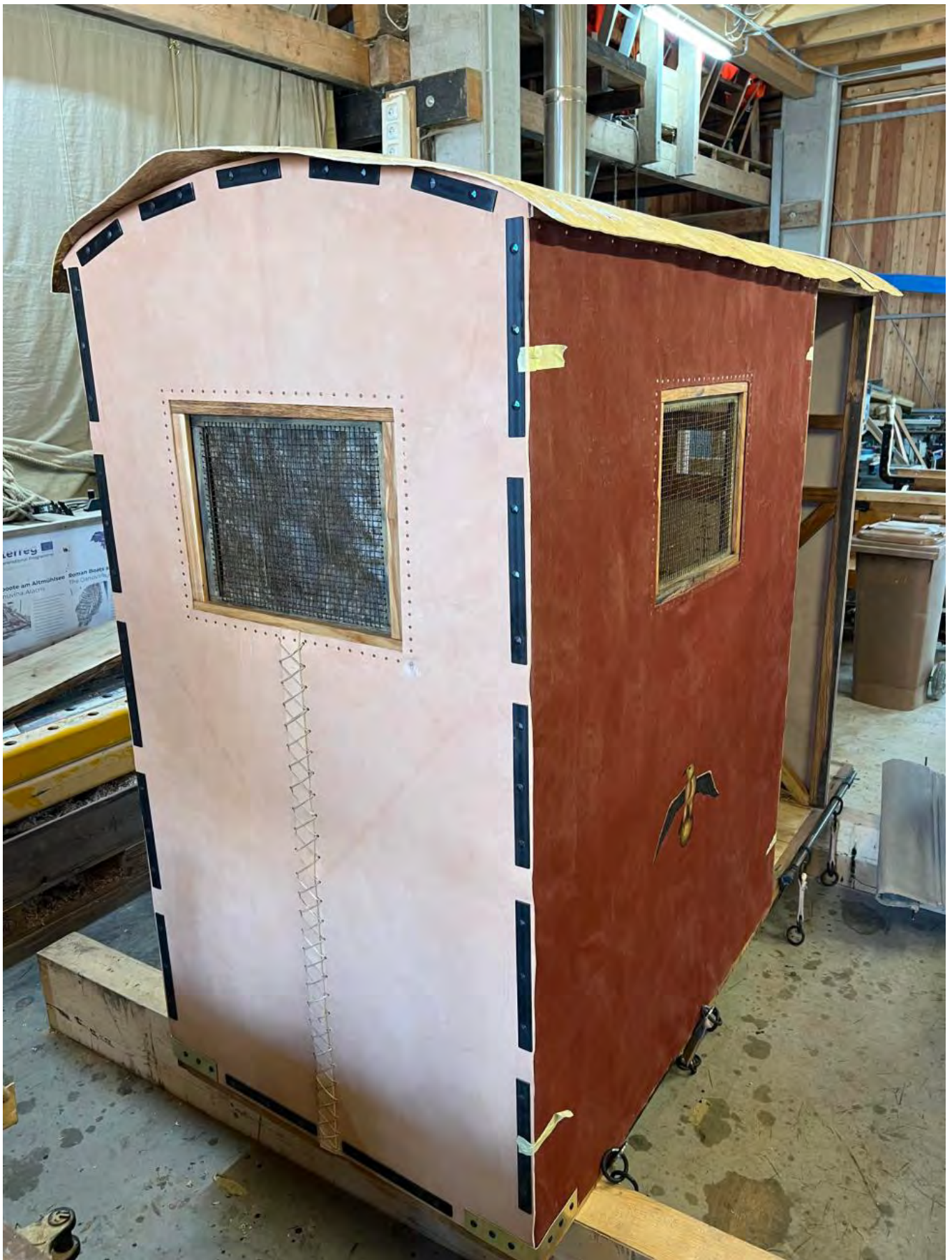
FIG 27. CARRIAGE BODY WITH ANTIQUE-PAINTED LINEN ON THE SIDES, LEATHER BACK AND FRONT WALLS, WITH TANNED COWHIDE LEATHER ROOF. PHOTO BY B. DREYER
