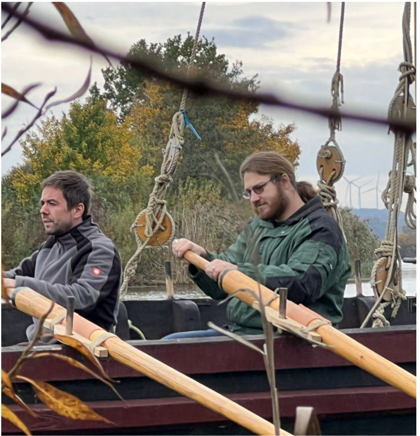
FIG 5A. THE DIFFERENT BELT SUSPENSIONS ARE SHOWN HERE, THE FIXED SUSPENSION OF THE OARS USED IN THE TESTS OF THE ROMAN BOAT RECONSTRUCTIONS CALLED VICTORIA AND RHENANA). PHOTO BY B. DREYER
