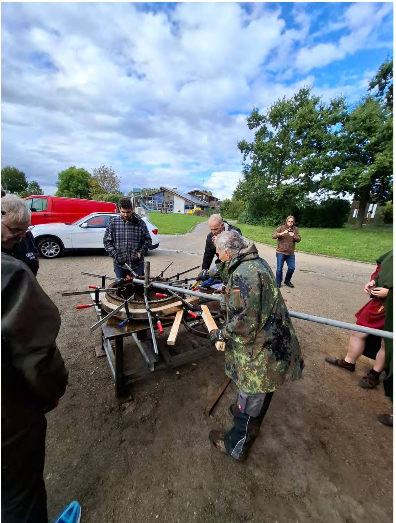
FIG 21. ONE OF THE MANY BENDING TESTS AFTER BOILING THE ASH PLANK FOR OVER 12 HOURS. PHOTO BY B. DREYER
