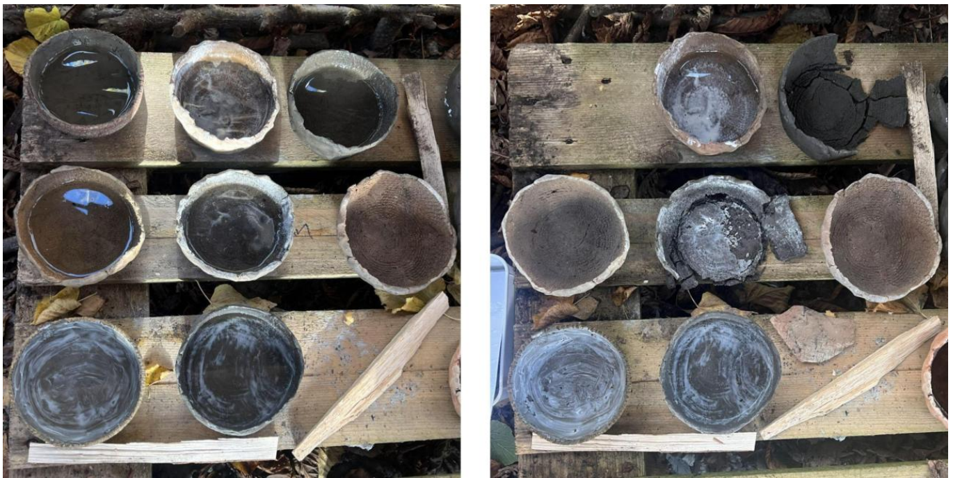
FIG 9. A SIDE BY SIDE OF THE POTS AT THE BEGINNING OF THE WATER RETENTION TEST (LEFT) AND AT THE END (RIGHT) AFTER 1 WEEK. PHOTOS BY TORTI, 2025
