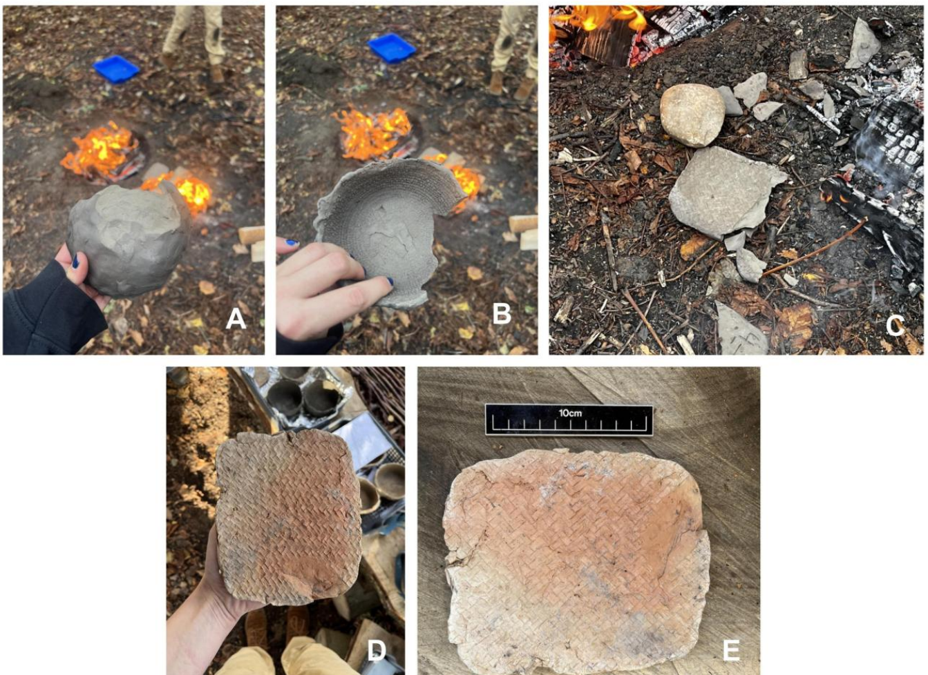
FIG 10. EXAMPLES OF SUCCESSFUL AND UNSUCCESSFUL FIRING. A AND B, A SPALLED CLAY VESSEL. C, A SPALLED HEARTHPLATE. D AND E, HP1, THE SUCCESSFULLY FIRED HEARTHPLATE WITH ONLY MINIMAL CRACKING AND SPALLING. PHOTOS BY HASSAN, O'CONNELL, TORTI, 2025
