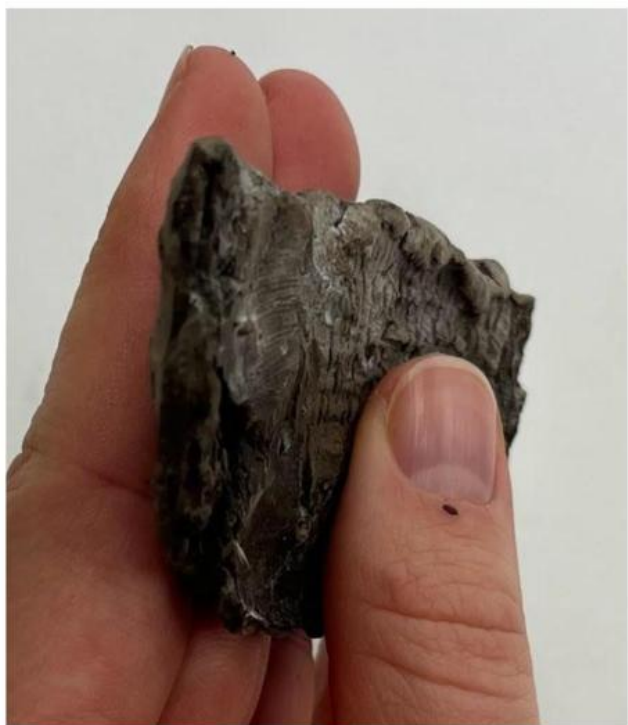
FIG 12. PHOTOS OF THE FRAGMENTS OF V7, THE EXPERIMENTALLY CREATED LEATHER HARD, UNFIRED, VESSEL WITHOUT A LINING OF ANIMAL FAT. THESE SECTIONS FELL AWAY DURING THE WATER RETENTION TESTS AND LOST A SIGNIFICANT AMOUNT OF CURVATURE DUE TO THEIR WATER LOGGED STATE. PHOTOS BY HASSAN, O'CONNELL, TORTI, 2025
