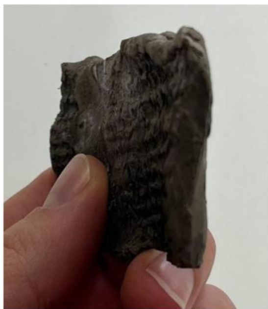
FIG 12. PHOTOS OF THE FRAGMENTS OF V7, THE EXPERIMENTALLY CREATED LEATHER HARD, UNFIRED, VESSEL WITHOUT A LINING OF ANIMAL FAT. THESE SECTIONS FELL AWAY DURING THE WATER RETENTION TESTS AND LOST A SIGNIFICANT AMOUNT OF CURVATURE DUE TO THEIR WATER LOGGED STATE. PHOTOS BY HASSAN, O'CONNELL, TORTI, 2025
