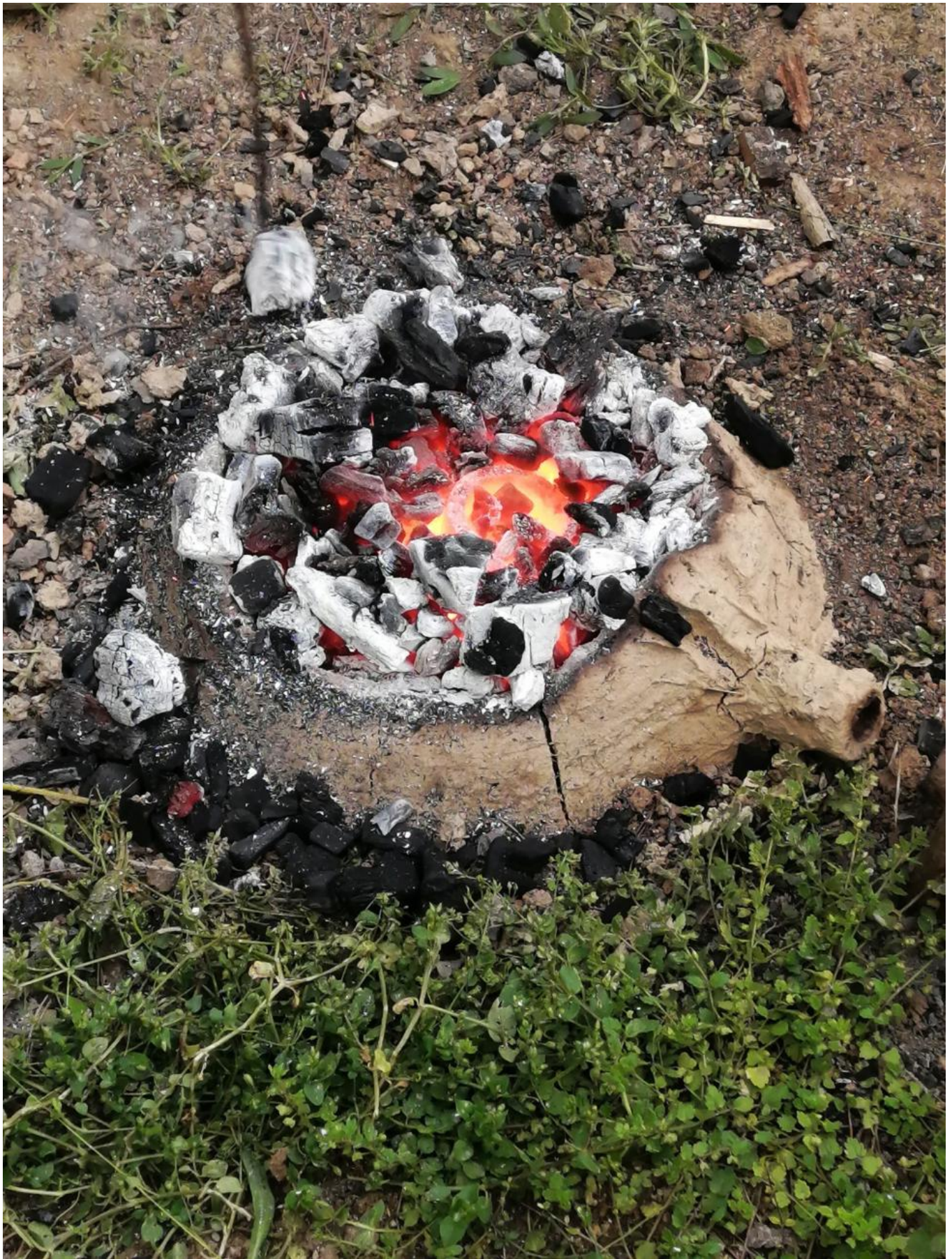
FIG 8. FURNACE AFTER DRYING AND PREHEATING WITH CHARCOAL. PHOTO BY DAMIAN JIROUT
