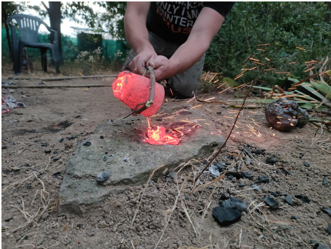
FIG 15. POURING MOLTEN COPPER FROM THE CRUCIBLE. PHOTO BY FILIP ŠEVČÍK
