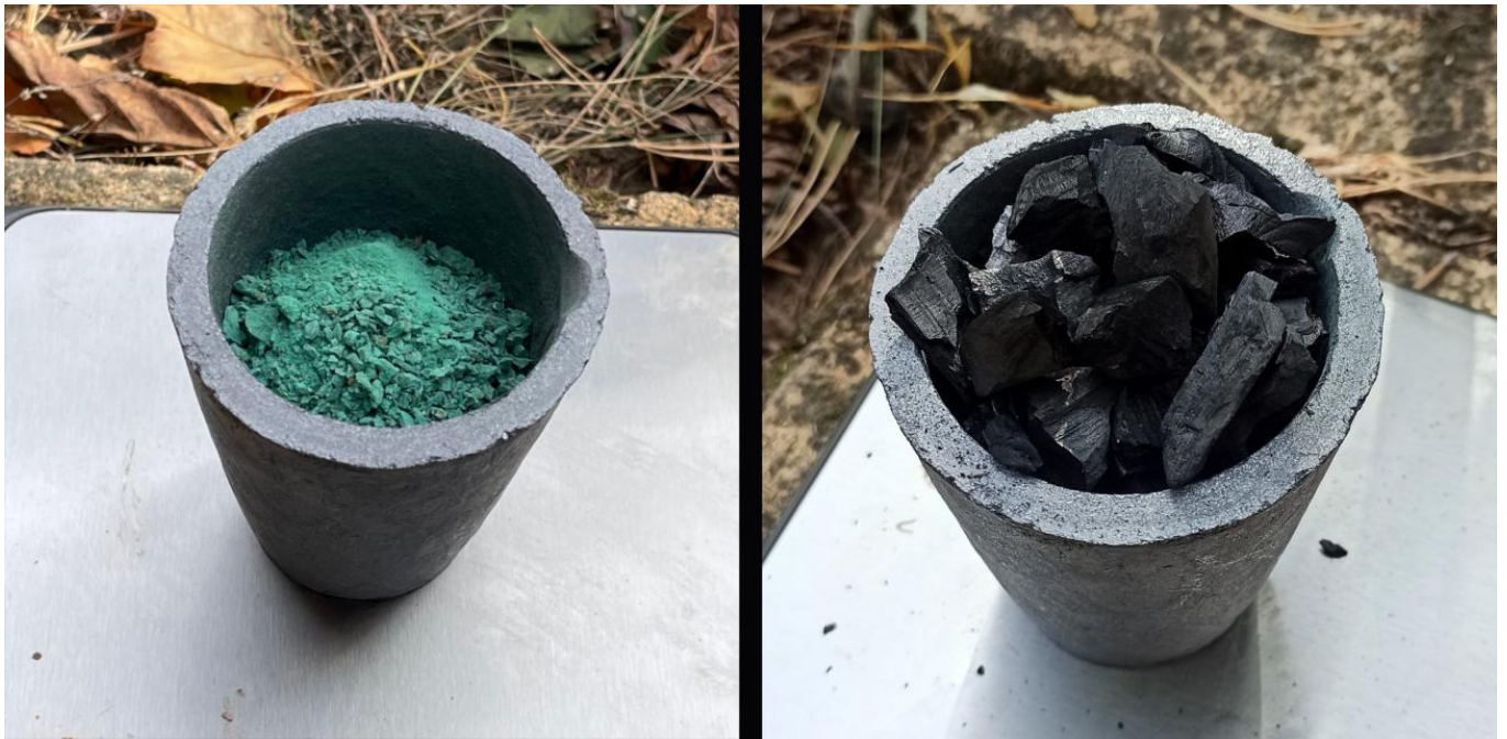
FIG 13. FILLING OF THE CRUCIBLE WITH ORE AND CHARCOAL. PHOTO BY VLADIMÍRA LEPLTOVÁ (1) AND ADAM PROCHÁZKA (2)
