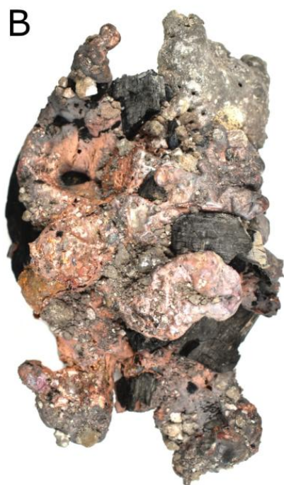
FIG 19. SELECTION OF COPPER LUMPS FROM THE FIRST PHASE OF EXPERIMENTAL SMELTS: A – CRUCIBLE SMELTS; B – DIRECT FURNACE CHARGE; C – SMELTS IN CLAY BALLS. PHOTO BY FILIP ŠEVČÍK
