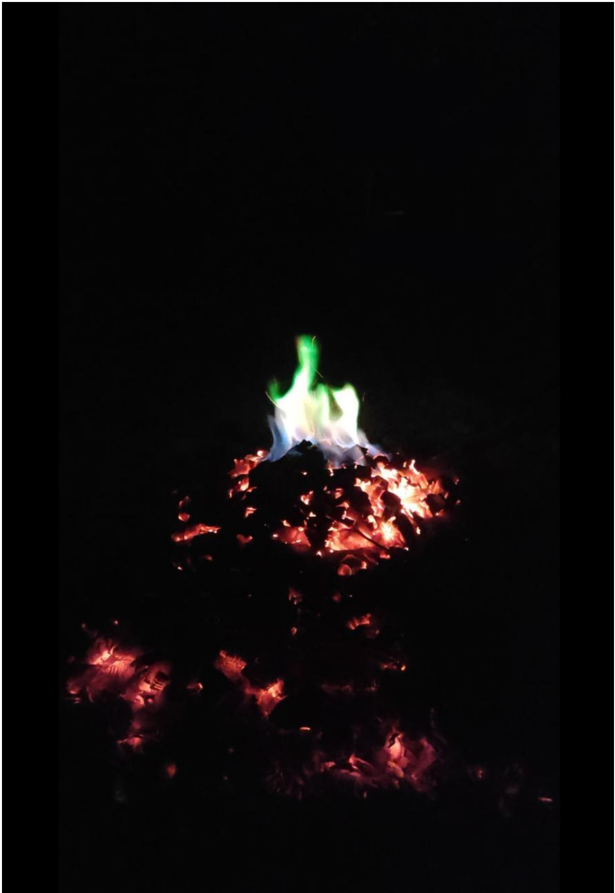
FIG 18. GREEN FLAME PRODUCED DURING DIRECT CHARGING OF ORE INTO THE FURNACE. PHOTO BY FILIP ŠEVČÍK
