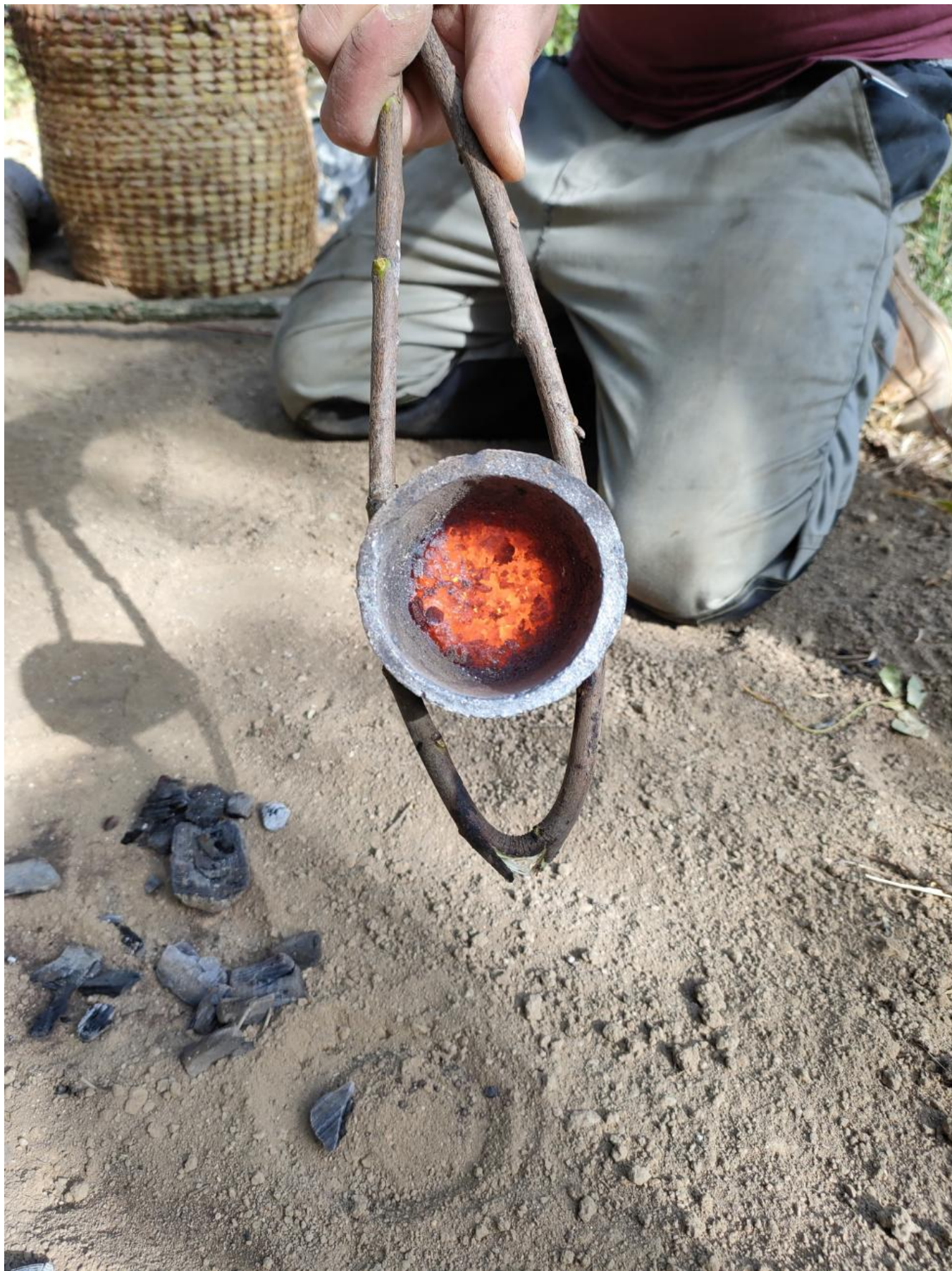
FIG 14. PARTIALLY REACTED CHARGE INSIDE THE CRUCIBLE. PHOTO BY FILIP ŠEVČÍK
