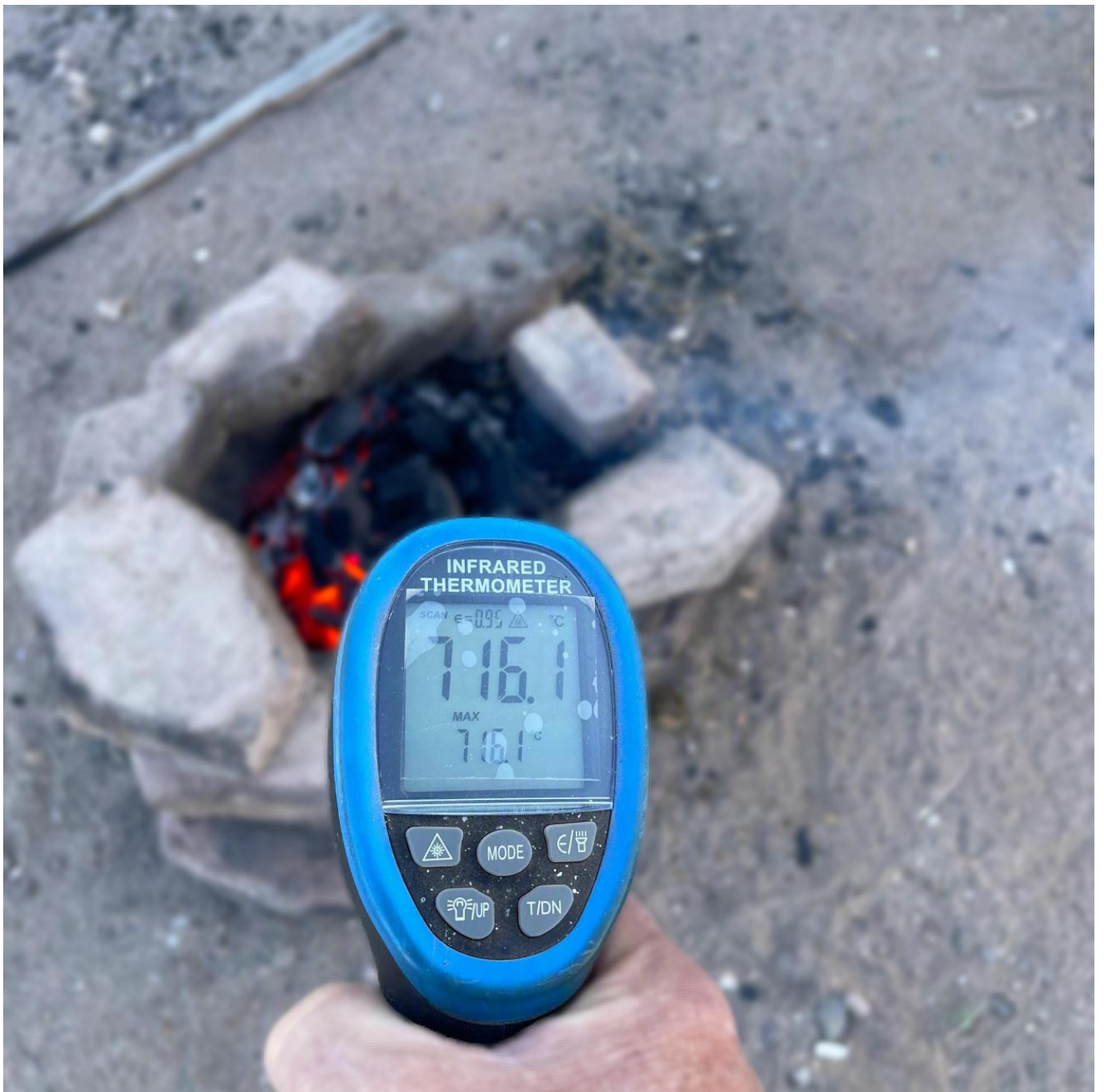
FIG 9. TEMPERATURE REACHING 716C ONSIDE OF BEAKER WITH COVER BOWL. PHOTO BY JEFF COOPER.
