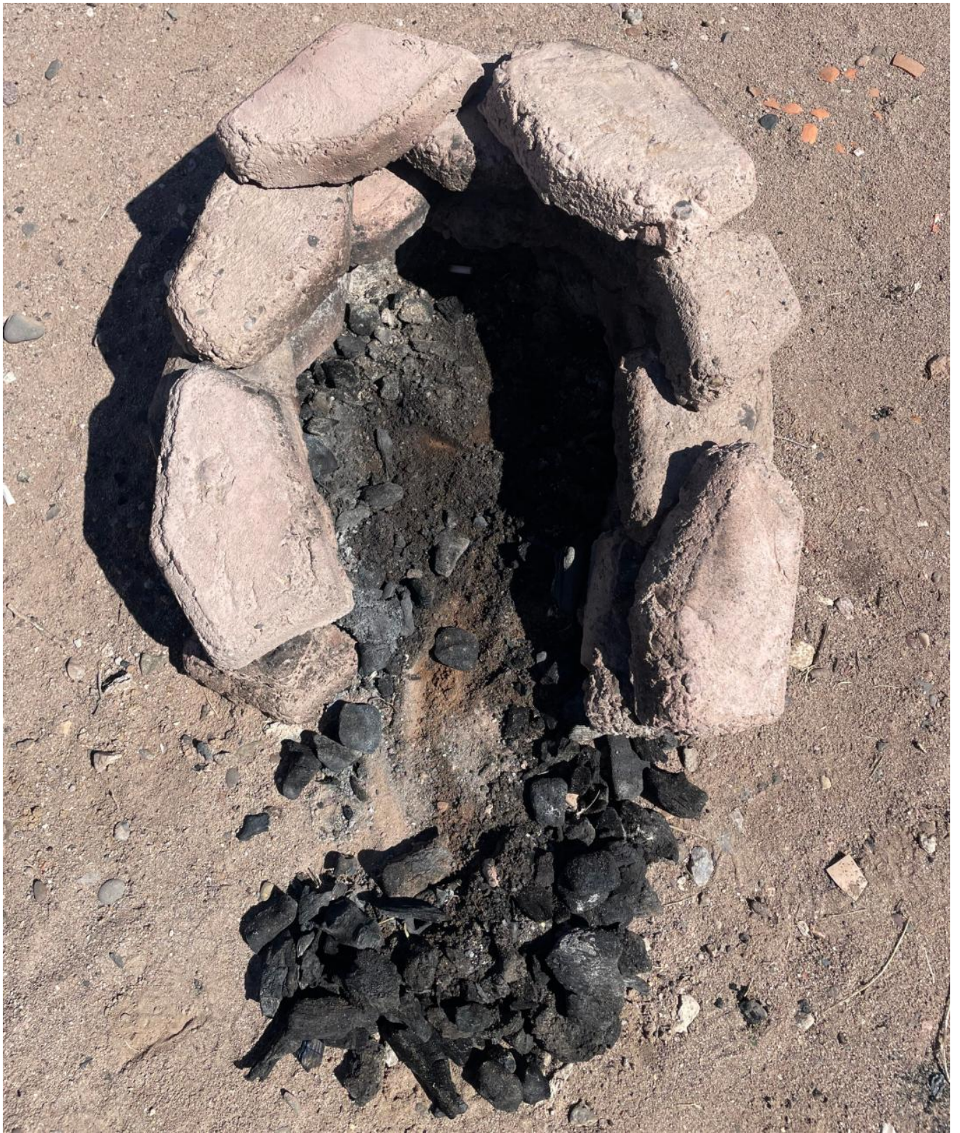
FIG 4. MY SIMPLE KILN WHERE I TEST FIRE KERMA BLACKTOP REDWARE. PHOTO BY JEFF COOPER
