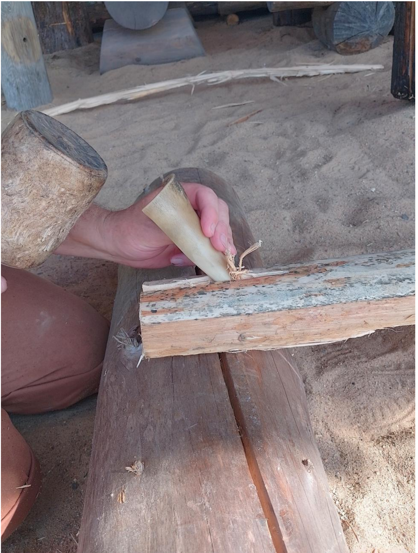
FIG 9. THE GEOMETRY OF THE BEVELLED BONE TOOL TENDED TO CAUSE TOOL RUNOUT. PHOTO BY WOODLAND, 2025
