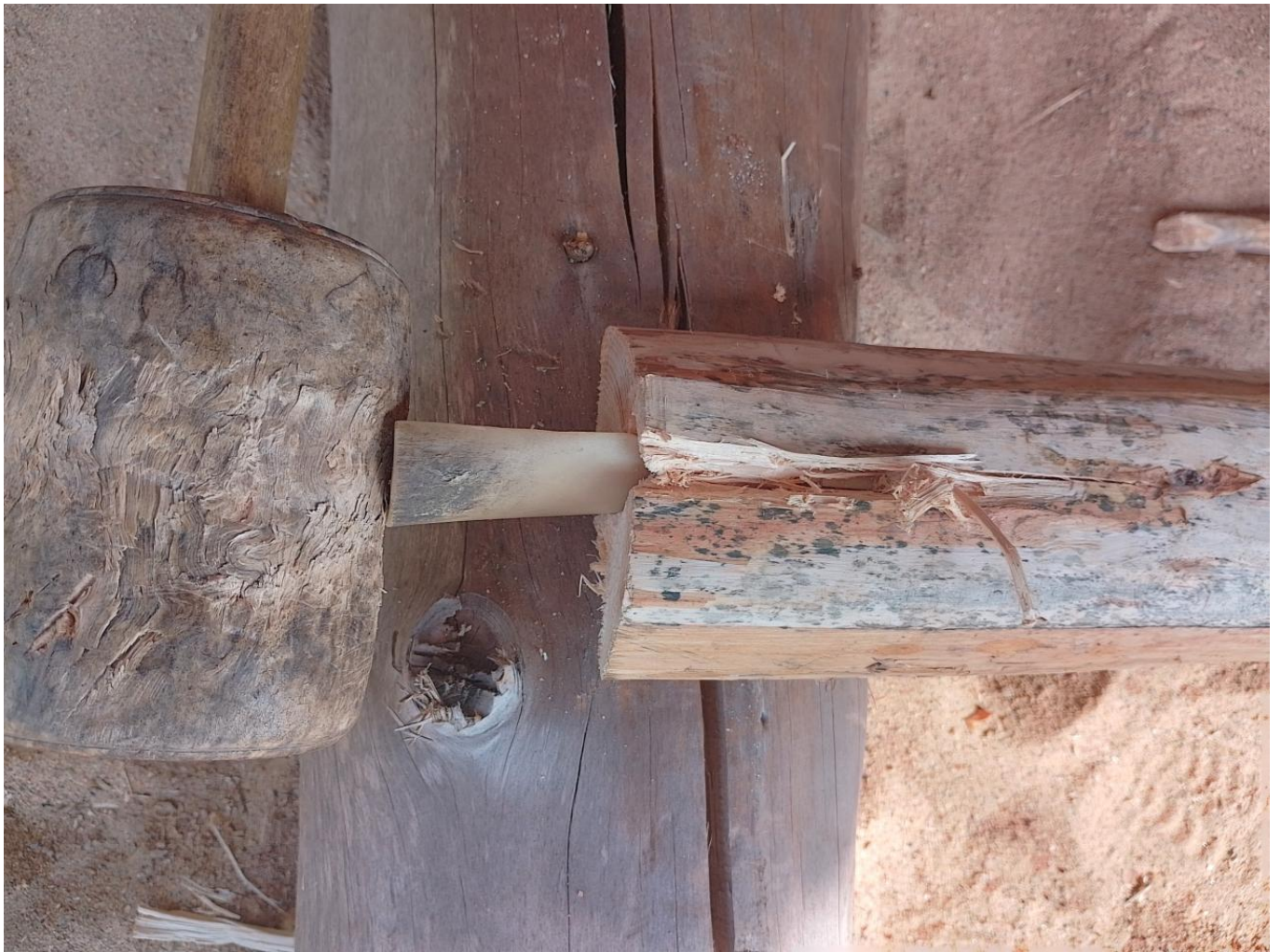
FIG 6B. CREATING A ROW OF INDENTATIONS WITH THE 45 DEGREE BEVELLED TOOL HELPED INITIATE THE SPLIT. B: SPLITTING ALONG THE INDENTATIONS. PHOTO BY WOODLAND, 2025
