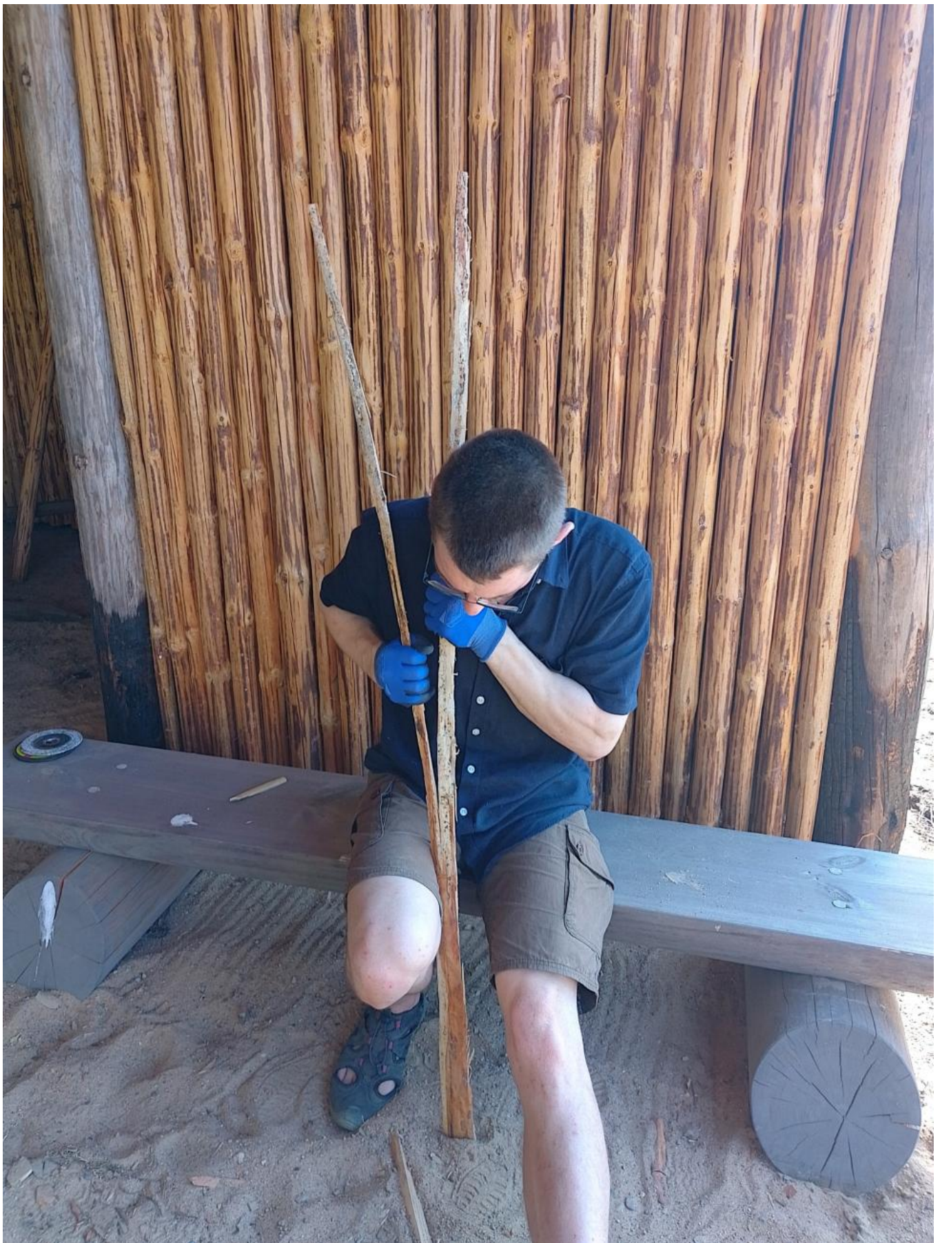
FIG 11B. ONCE THE SPLIT IS INITIATED BETWEEN INDIVIDUAL LATHS USING A BONE TOOL THEY ARE PRIMARILY CAREFULLY SPLIT BY HAND USING VARIOUS LEVERING TECHNIQUES TO KEEP THE TWO INDIVIDUAL LATHS EVEN. B: "CHASING" THE SPLIT TO THE BASE. PHOTO BY GROOM, 2025
