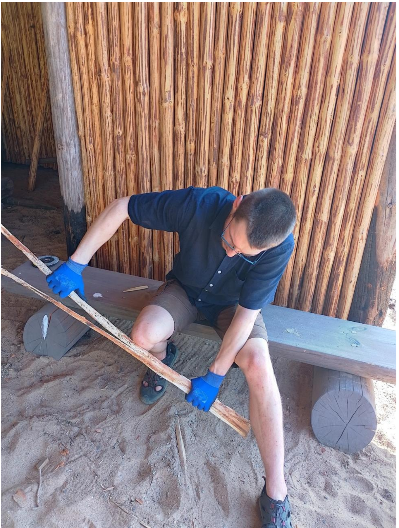
FIG 11C. ONCE THE SPLIT IS INITIATED BETWEEN INDIVIDUAL LATHS USING A BONE TOOL THEY ARE PRIMARILY CAREFULLY SPLIT BY HAND USING VARIOUS LEVERING TECHNIQUES TO KEEP THE TWO INDIVIDUAL LATHS EVEN. C: USING KNEE LEVER TO KEEP THE SPLIT RUNNING EVENLY. PHOTO BY GROOM, 2025
