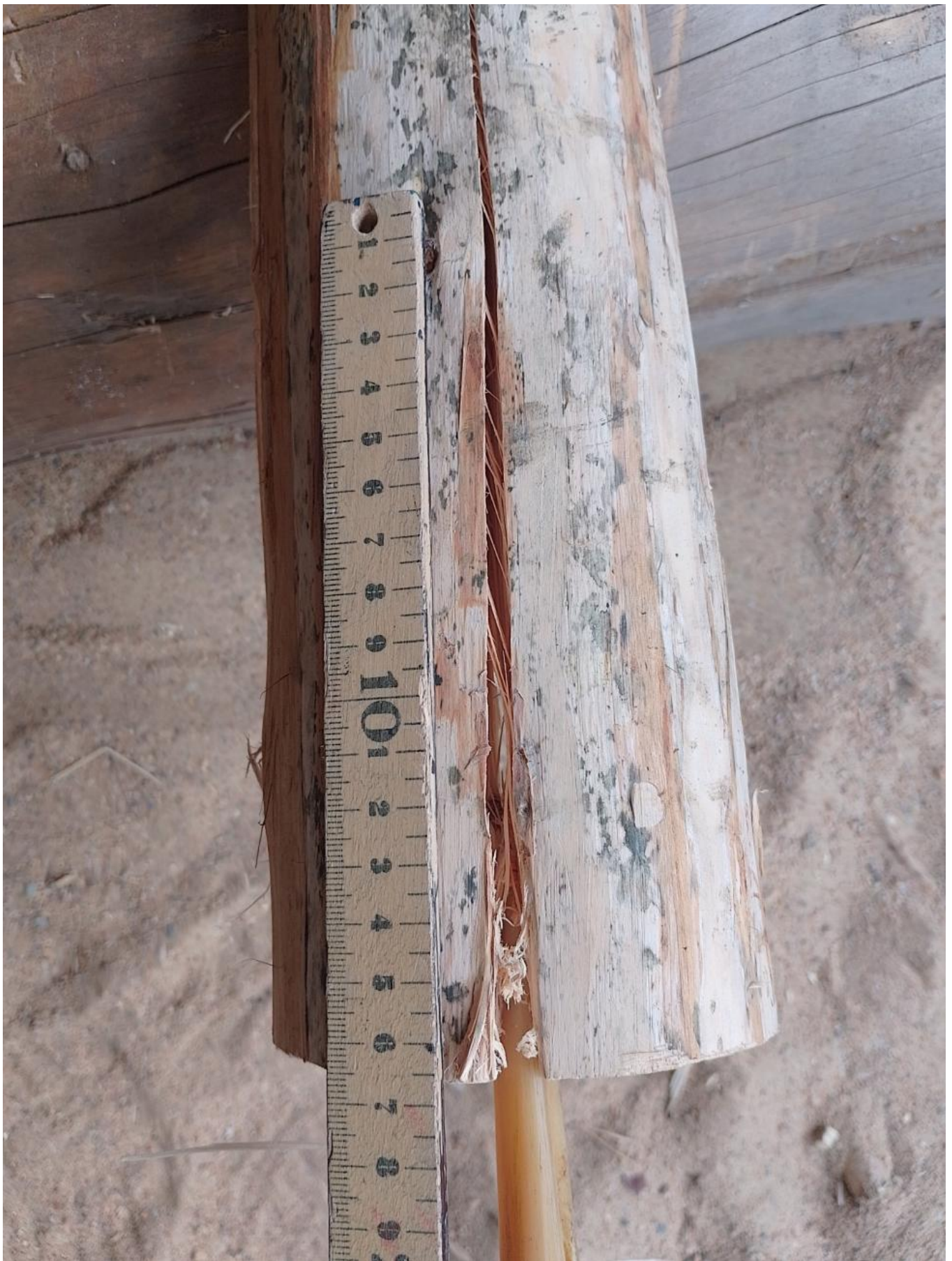
FIG 13B. THE INTUITIVELY DEVISED BONE SPLITTING WEDGE HAD A BEVEL WITH GEOMETRY WELL SUITED TO SPLITTING. B: THE LOG SPLIT EVENLY AND EASILY. PHOTO BY WOODLAND, 2025
