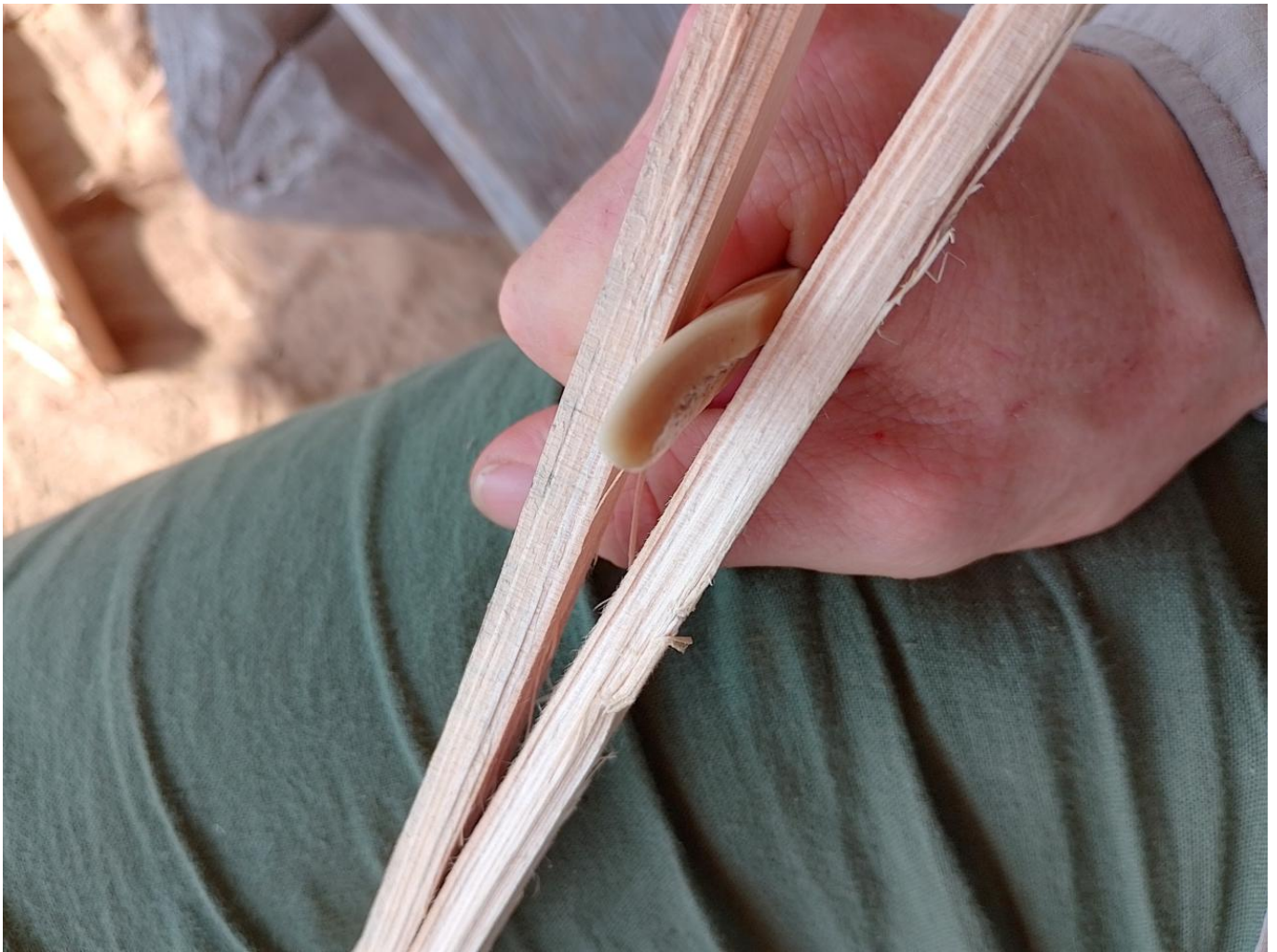
FIG 11A. ONCE THE SPLIT IS INITIATED BETWEEN INDIVIDUAL LATHS USING A BONE TOOL THEY ARE PRIMARILY CAREFULLY SPLIT BY HAND USING VARIOUS LEVERING TECHNIQUES TO KEEP THE TWO INDIVIDUAL LATHS EVEN. A: INITIATING THE SPLIT. PHOTO BY GROOM, 2025
