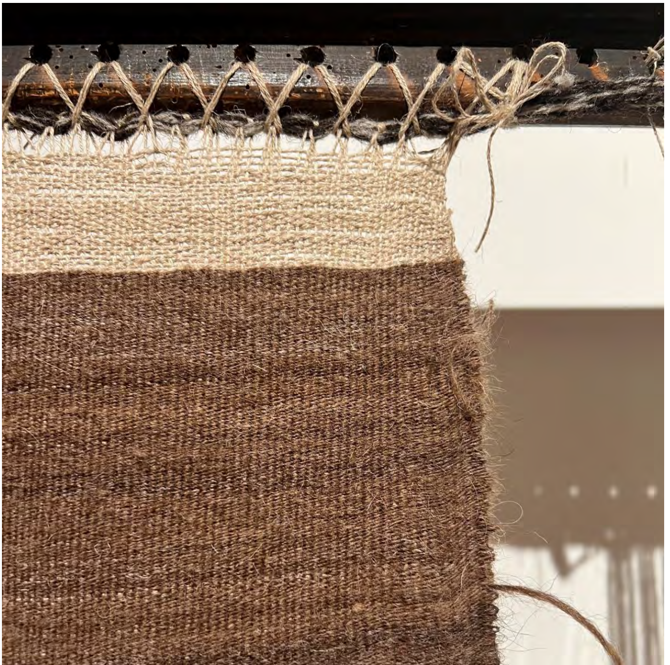
FIG 9A. THE RESULTS OF REUSED THREADS FROM WOVEN TEXTILES: A – WOOL THREAD WITH LINEN WARP. PHOTO BY M. RAVNANGER
